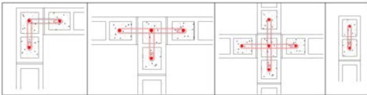
FIGURE 10 - REBAR TIES (R6@400) AT WALL JUNCTIONS AND END
